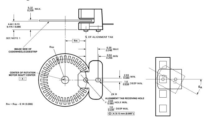
For linear motion, angular misalignment,  $E_A$ , must be  $\leq \pm 2$  degrees to achieve Encoding Characteristics.
